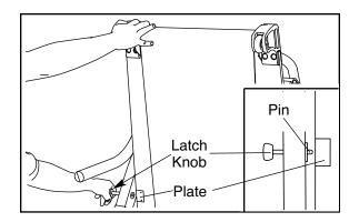
Hold the treadmill firmly with both hands, and lower the treadmill to the floor. Do not drop the treadmill frame to the floor. CAUTION: To decrease the possibility of injury, bend your legs and keep your back straight.
